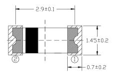
Suggested pad dimension is just for reference only. Please modify the pad dimension based on individual Note: Tolerances unless mentioned  $\pm 0.1$ mm. Unit = mm
