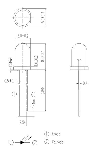
Note: Tolerances unless dimensions ±0.25mm
