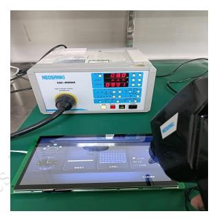
Electrostatic discharge test
