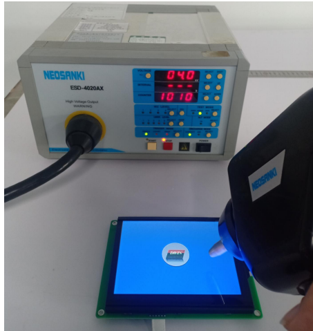
3.1 Electrostatic discharge test
